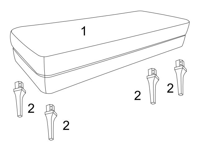
STEP 1: Attach Legs (2) to base frame (1), using flat washer (A), Lock Washer (D), and bolt(C) as shown below,, then tighten with allen key(B).
